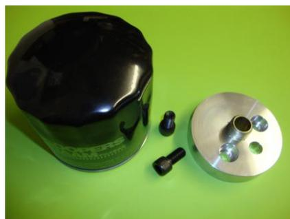
Examine the oil filter adaptor and compare it with the seating face on the engine block. The adaptor can only be fitted in one position (so that all the holes are in the lower half). You are advised to use sealing compound or gasket paper between the adaptor and the block. Fit the adaptor using the bolts supplied, and tighten the bolts.
